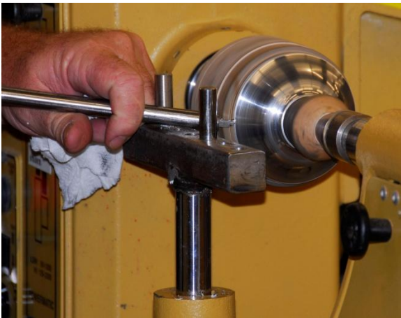
The top of the bowl is trimmed up using a trimming tool, a steel bar fitted with a 1/4" steel lathe cutting tool. Another shop made tool. [I found a box of five carbide tipped 1/4" cutting tools at Harbor Freight for around $5. JIG].
