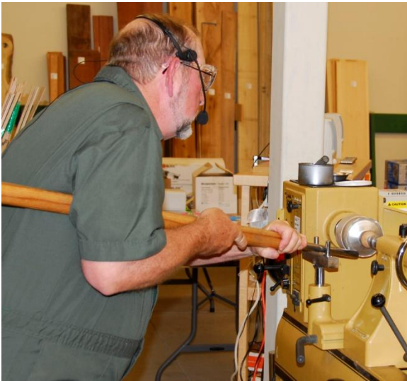
This shows Tom using the finger tool and tool rest to flow the metal down and around the mandrel.
