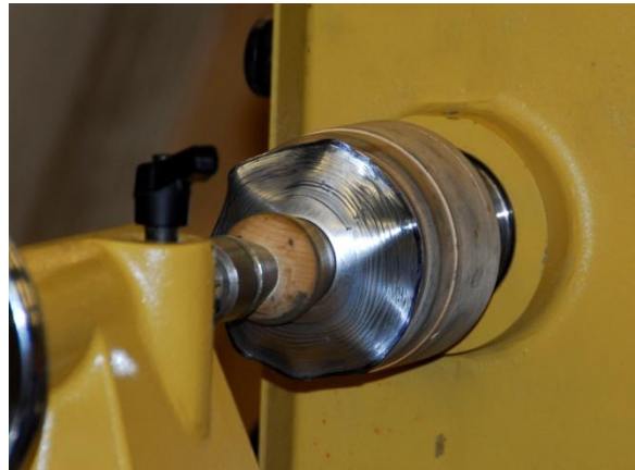
Too much pressure too far out on the mandrel can cause cockling (wrinkling of the metal). If the cockling is not too bad, the end of the finger tool can be used to lift up the edge and move it slightly back toward the tailstock. Then using a backing stick in your left hand, put it under the cockled metal and use the finger tool to iron out the wrinkles. Yes, you are using the backing stick in the left hand and the finger tool in the right hand at the same time. Both tools are across the toolrest prying against the pivot pins trying to iron out your mistake. And yes, you will be very busy at this time. If is not cockled too bad and if you are lucky (good) you will be able to salvage the work, otherwise start over.
