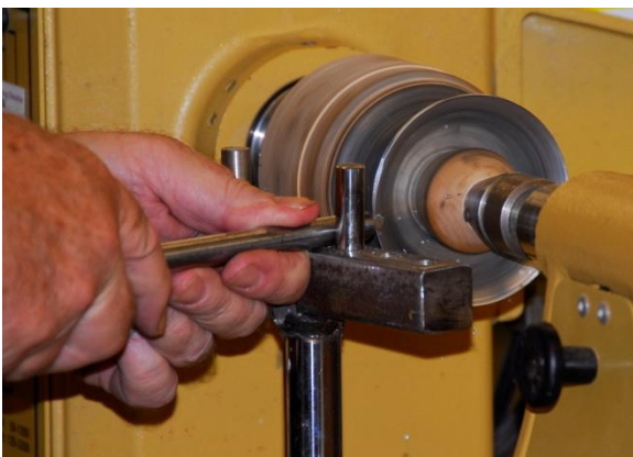
The bowl is then reversed and final trimming of the top is performed
