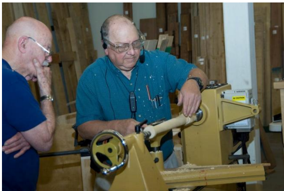
Figure 5. John is turning the taper while being watched by Doc.
