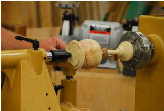
Figure 3. Shaping the base while mounted on special jam chuck.
