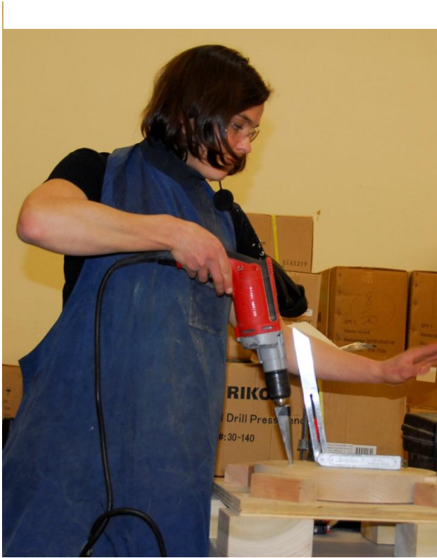
Figure 4 Using the sliding bevel to position drill.
