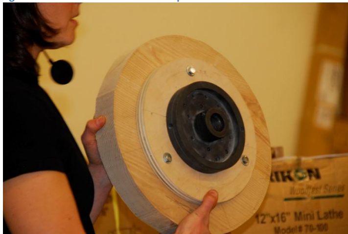
Figure 2 Seat blank mounted to faceplate.
