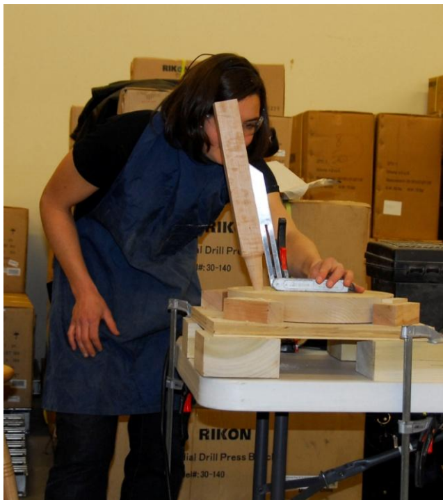
Figure 5 The sliding bevel verifying correct angle of test leg.
