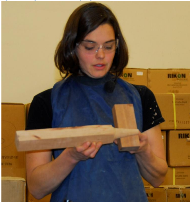
Figure 3 Megan shows how gauge block is used to size tenon on test leg.
