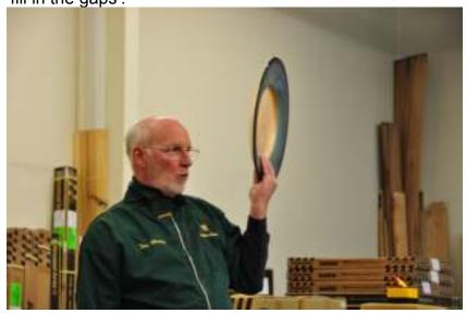
Tom used a maple blank about 2" thick that had been cut into a circular blank. Most blanks of this size are not perfectly flat but will be slightly warped or cupped. A faceplate is mounted on the most concave side. This will be the upper surface of the platter,
