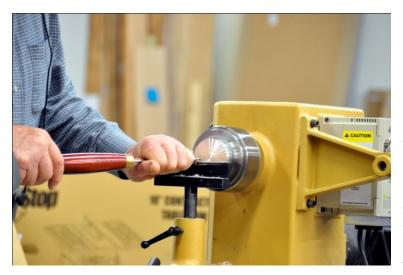
John mounted a pewter button on the lathe and demonstrated how to shape it using scrapers and other tools.
