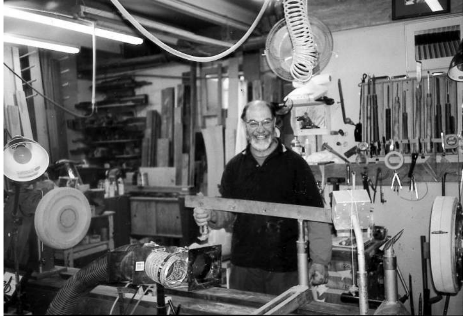
David Nittmann, a high-energy artist, at his 12-ft. Ullery/Nichols lathe. The large drum-like fixtures on the headstock and tailstock are for architectural work, a major component of his business. Photo by Ken Keoughan.
