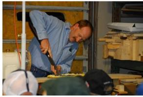
with a skew, Alan's favorite tool. Alan indicated that the skew is a very versatile tool when doing spindle turning and that you don't need little tools to make little turnings. To demonstrate this, he used his 1 3/8 inch skew to turn some very small tops. To make them easier to see and pass around, they were placed on the sticky side of a piece of black electrical tape. No one present, volunteered to test spin the tops. Note that there are two tops in the photo.
