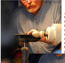
Alan used the skew for most of the turning done during the evening. I don't remember his using the grinder for sharpening, instead, he honed his tools using a Diamond Hone.
